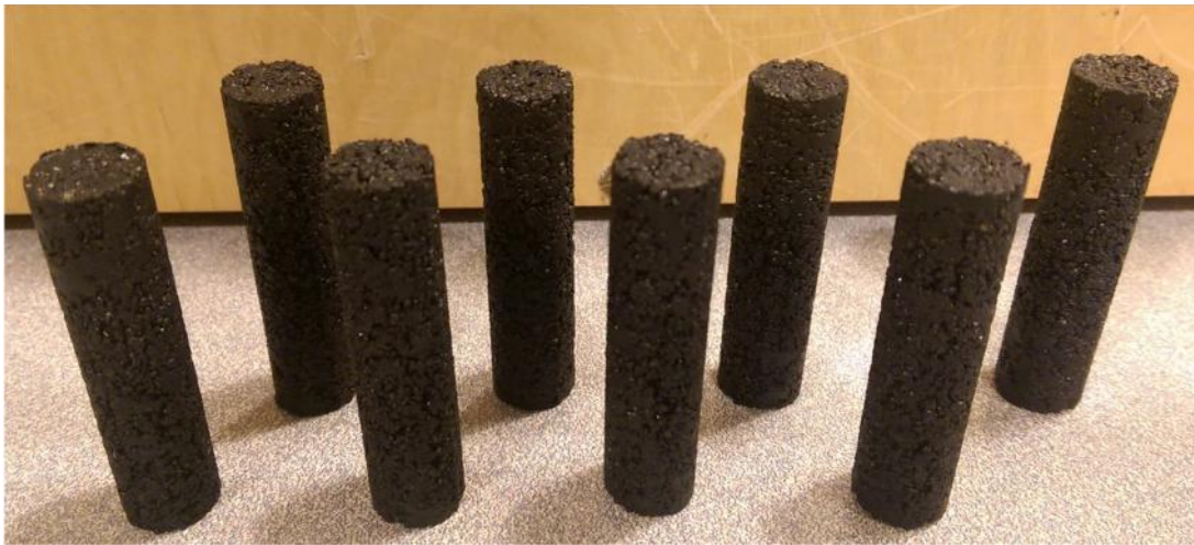
Figure 3.2. FAM specimens, 12 grams mass, 50 mm long with a 12 mm diameter.
