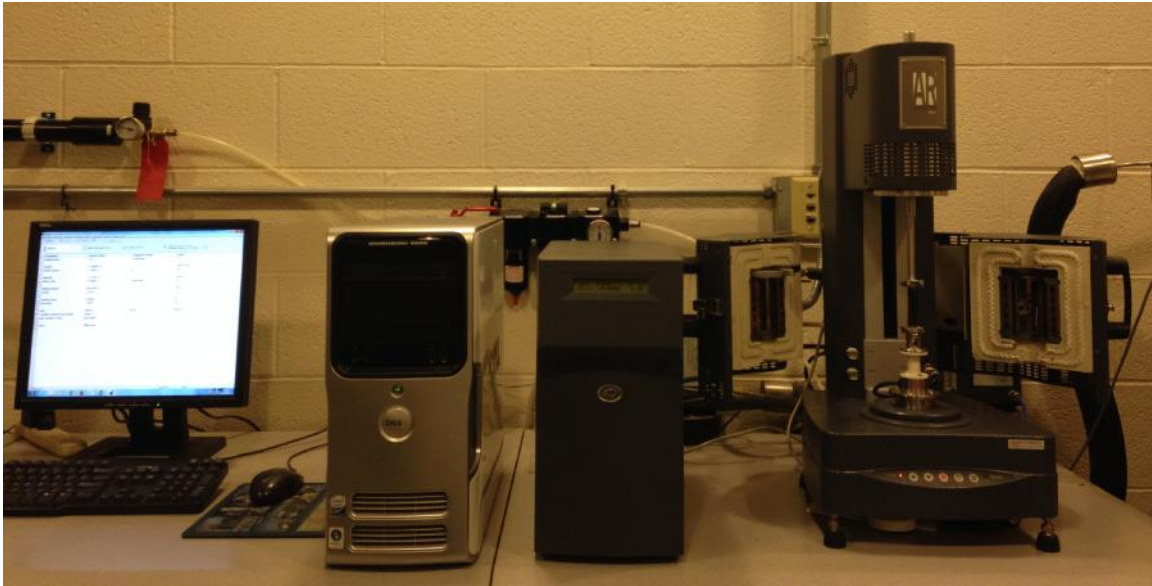
Figure 4.2. The dynamic mechanical analyzer, AR2000ex rheometer.
