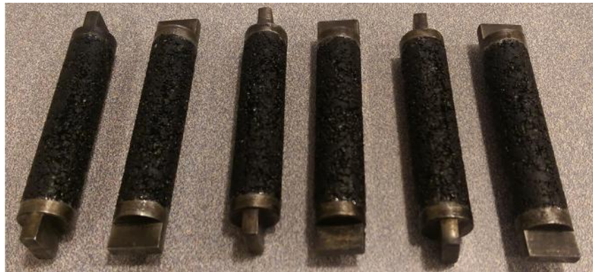
Figure 3.3. Fine aggregate matrix specimens with holders.
